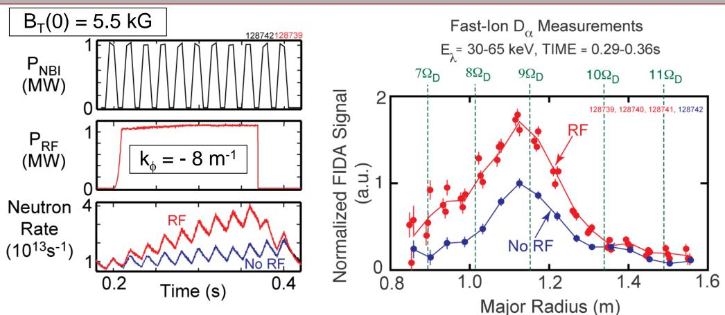
Measured acceleration of NBI fast-ions and large increase in neutron rate during HHFW + NBI plasmas
