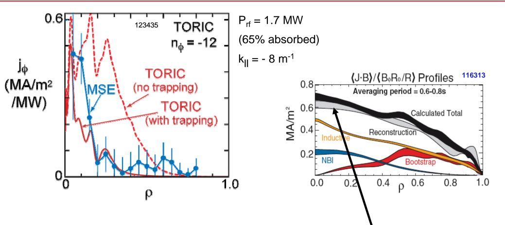
• High non-inductive fraction H-mode  $J_{\phi} \sim 0.5-0.7 MA/m^2$
